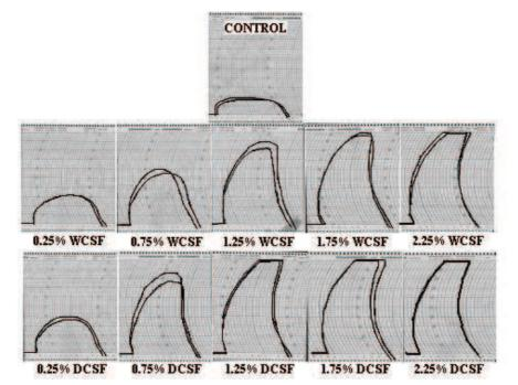
Fig. 2. Extensograms of wheat-wheat bran composite flour (control) containing CSP (WCSF and DCSF).
