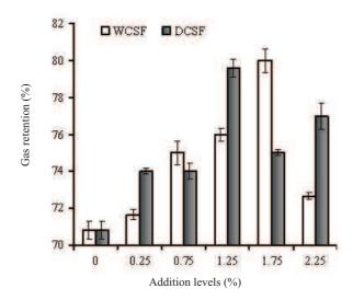
**Fig. 4.** Effect of WCSF and DCSF on gas retention of dough obtained from wheat-wheat bran composite flour.
